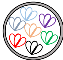
Figure 1A- Generic representation for a Flexi Duct in 100mm DWC Pipe (Sample)
